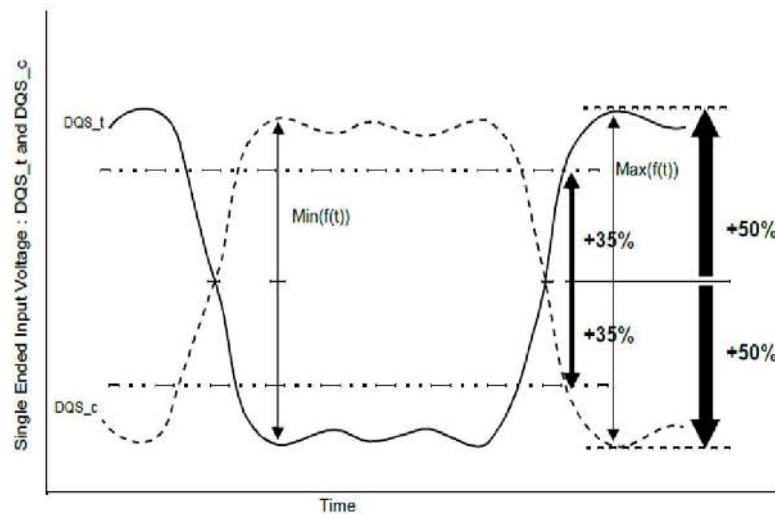
**Definition of differential DQS Peak Voltage and range of exempt non-monotonic signaling**
