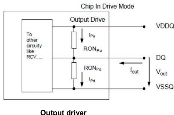
**Output Driver DC Electrical Characteristics, assuming RZQ = 240ohm; entire operating temperature range; after proper ZQ calibration**
