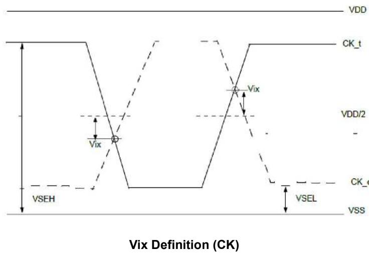
**Cross point voltage for differential input signals (CK)**
