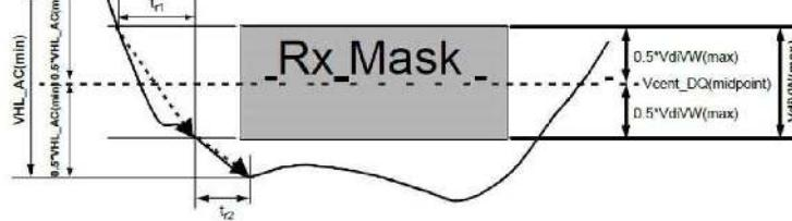
**Slew Rate Conditions For Falling Transition**
